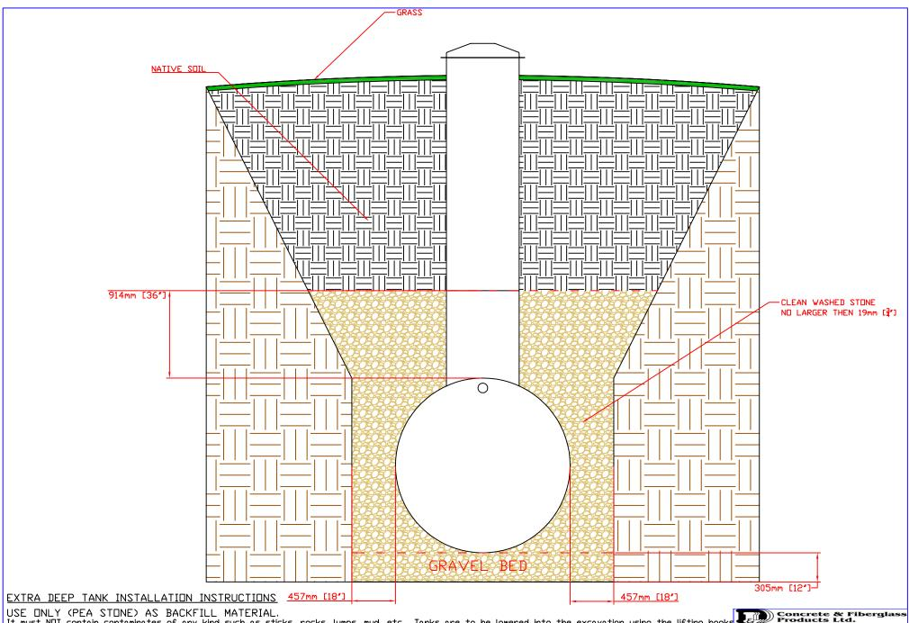
It must NOT contain contaminates of any kind such as sticks, rocks, lumps, mud, etc. Tanks are to be lowered into the excavation using the lifting hooks on the tank. Tanks must NOT be buried deeper then the tank label indicates, measuring from the top of the tank to the finished ground level.
